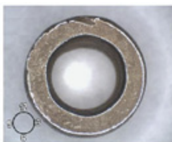
Figure 1: A crack in a self-locking nut observed on a nut, (detail view).
