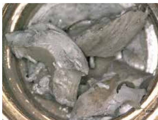
Figure 2. Fuel selector valve housing and section of selector handle (left) and fuel selector insert with fractured pieces (above).
