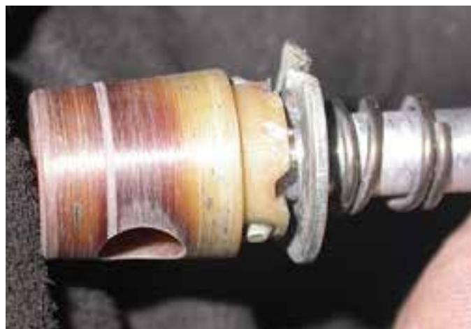
Figure 5. Plug cock showing discoloration, scoring, wear, debris, and a worn detent.
